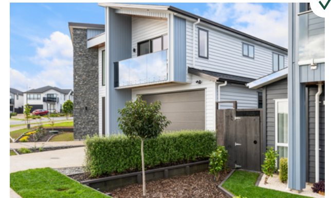
The front yard boundaries of these homes are defined with low height hedging, and the side fence does not protrude from the corner of the house.
